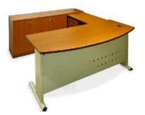
Table of an overall size 1200x600x750 with top made of 25mm thick Prelam Particle Board having Radial profile in front side. The table understructure has vertical leg made of 1.2mm CRCA double walled legs with triangular shape foot and top duly powder coated with ABS caps at ends. The modesty is made of 1.0mm CRCA sheet having perforation design in it duly powder coated. All the exposed edges sealed with 2mm PVC edge banding tape pressed at 2000 C with hot melt glue on special machines.
