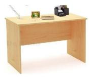
Table of an size 1200W x 600D x 750Hmm with top made of 25mm thick plain particle board having 0.6mm post formed decorative laminate on top and balancing laminate on unexposed face. The understructure is made of 18mm thick prelaminated particle board with all exposed edges sealed with 2mm PVC edge banding tape and all unexposed edges sealed with 0.6mm edge banding tape pressed at 2000 C with hot melt glue on special machines. Table has a provision for wire manager caps at top.
