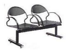
**Multiseater chair** with perforated metal sheet duly powder coated with arms in capsule pipe, side in 2" round pipe and bottom support in 3" x 1/2" in 14 gauge.
