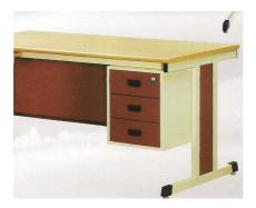
Providing & fixing Free standing workstation table of an over all sizes 2100x2400x600 for each person with Top made up of 25mm Prelaminated MDF board having decorative laminate 0.8mm on top and balancing laminate on unexposed face, All exposed edges are sealed with 2mm PVC edge banding pressed at 200o C with hot melt glue on special machines. The worktop is supported with CRCA Powder Coated Steel Legs. (W/O KBPT/CPU/DRAWER UNIT)
