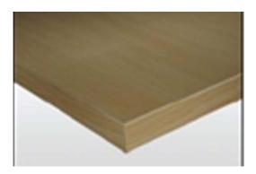
Providing & fixing Work Top made up of 25mm thick prelaminated particle board having decorative laminate on top and balancing laminate on unexposed face, All exposed edges are sealed with 2mm PVC edge banding pressed at 2000 C with hot melt glue on special machines. The worktop is supported with cantiliver brackets made of MS steel duly powder coated. Worksurface is also provided with ABS wire manager of 50mm dia.
